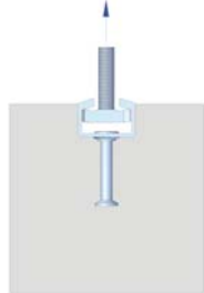
Breakout of channel lips under tensile loading
