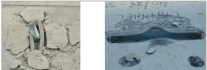
Breakout of T head bolt under shear loading
