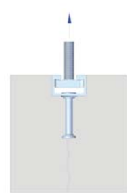
Splitting of concrete under tensile loading
