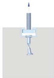
Breakout of stud under tensile loading
