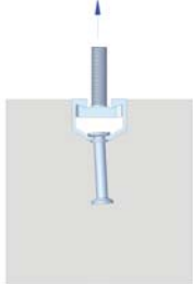
Breakout of channel stud under tensile loading
